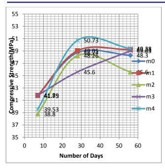
The results for sulphate resistance of concrete showed that the compressive strength of concrete was decreased by 3% in case of control mix and 3-7% in case of RCA concrete. At the age of 56 days, compressive strength of m4 was reduced to 92.75%.
