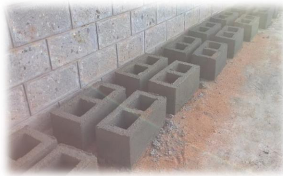
Plate 4:-Blended Sandcrete Blocks containing Sugarcane Bagasse Ash.
