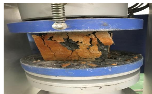
Figure 3: Compressive strength test after acid attack
