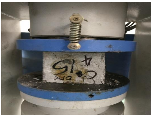
Figure 1: Compressive strength testing
