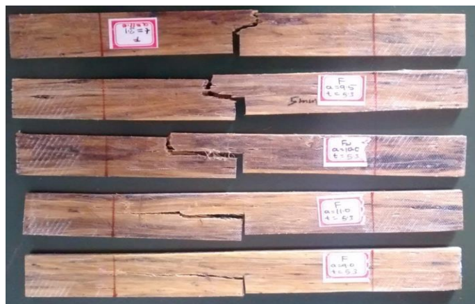
Fig 5. Tested Single Edge Notched Tensile (SENT) specimens
