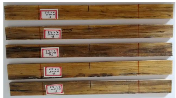
Fig 3. SENT specimen of Hemp fiber composite
