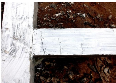
Figure 3. Failure pattern of HPC beam column joint subjected to cyclic loading
