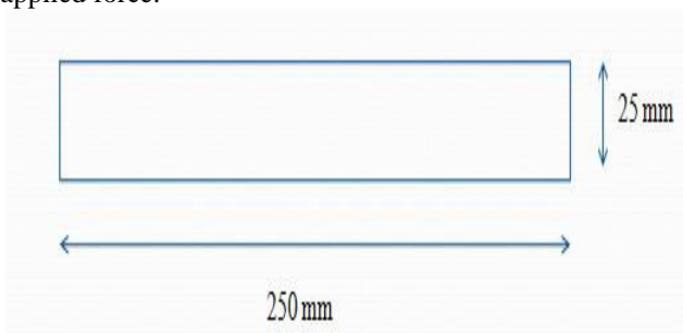
Fig 3: tensile test specimens as per ASTM D3039-76 standards
