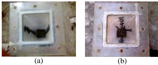
Fig. 2 Fluidized bed dryer column (a) without spirals (b) with spirals
