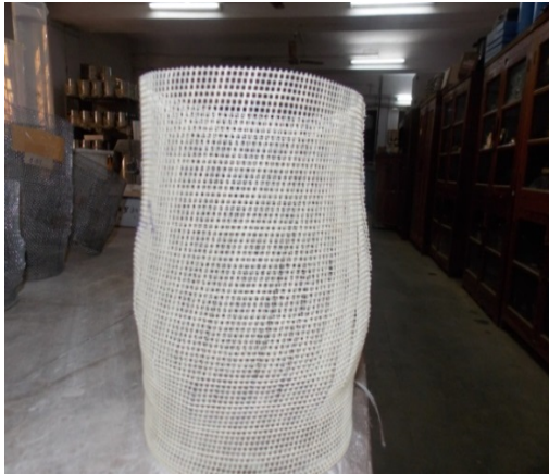
Fig. 5. Deformed shape of encasement of ESC: (a) for l/d = 0.5 ; (b) for l/d = 1 .
