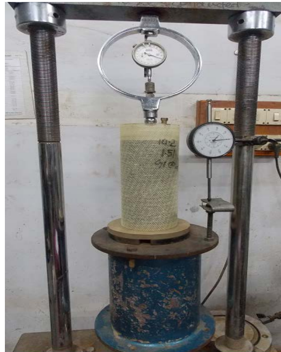
Fig. 2. Encased SC under the loading frame.
