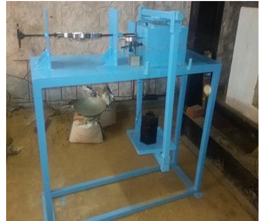
Fig 2 Large Scale Direct Shear Test
