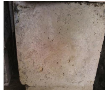
Photo 3 Cube after removing from Sulphate Solution
