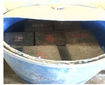
Photo 2 Specimen's immersed in Sulphate Solution
