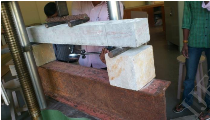
Figure 3: Two point load test on beams
