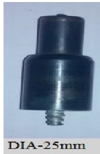
Fig. 3 FSW tool with threaded tip
