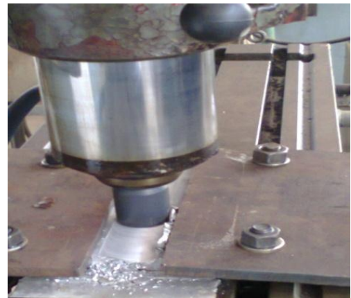
Fig. 5 FSW experimental Set-up
