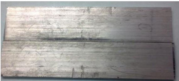
Fig. 4 working AL-plates to be welded
