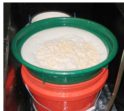
Fig. 2. Screening the contents of the ball mill to recover the collagen nanofibrils
