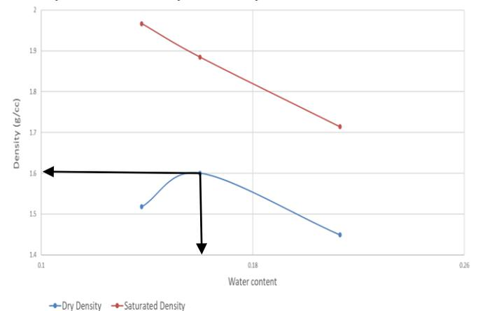
Fig 1- Compaction curve of 0.5% polypropylene fibers on soil From the graph, the dry density will be increases up to a
