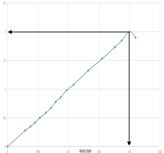
Fig 5- Axial stress-strain graph of 1% polypropylene fibers on soil
