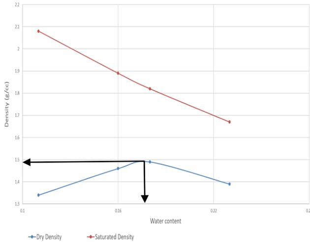
Fig 3- Compaction curve of 1.5% polypropylene fibers on soil. From the result, the dry density will be increases up to a limit and then decreases which shows the compaction curve. This curve reveals that the maximum dry density is obtained as 1.49 g/cc and optimum moisture content as 18 %.
