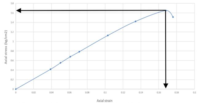
Fig 4- Axial stress-strain graph of 0.5% polypropylene fibers on soil
