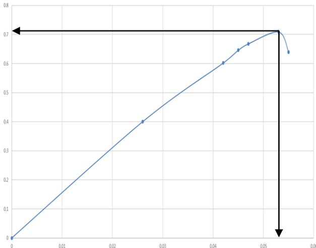
Fig 6- Axial stress-strain graph of 1.5% polypropylene fibers on soil
