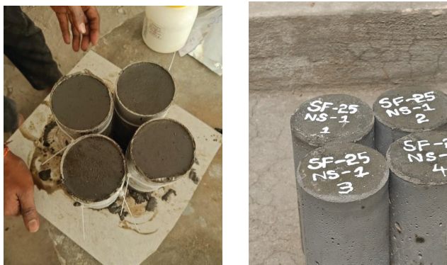
Fig.8,9 Casting & Curing of Specimens
