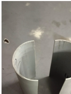
Fig.7 Prepared Mould [Dia-72mm, Depth-144mm]
