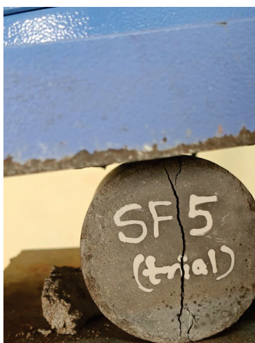
Fig.11 Crack Formed in the Specimen
