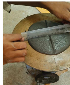
Fig.10 Flow Table Test
