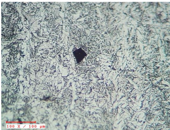
Fig. 3. Weld Zone Microstructure of Flux-Coated Workpiece
