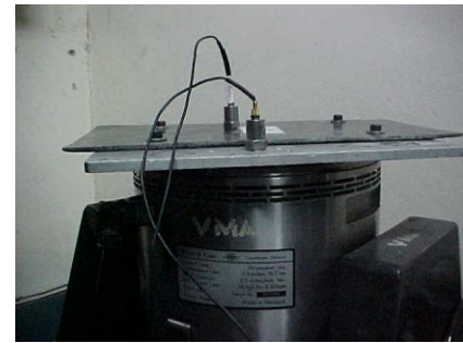
Fig: a composite plate placed on vibration exciter 4809
