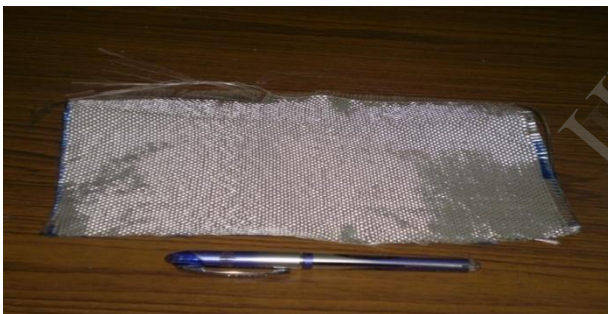
Fig: Bi directional s-glass woven fiber
