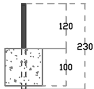
Fig 4. Test Specimens detailing
