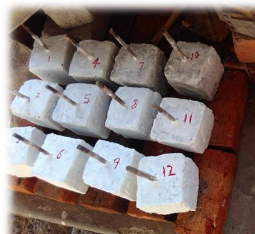
Fig 3. Test Specimens after final capping
