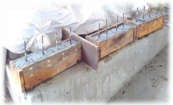
Fig 2. Casting of Specimens
