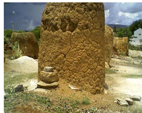
Fig.1: Local lime-burning kilns
