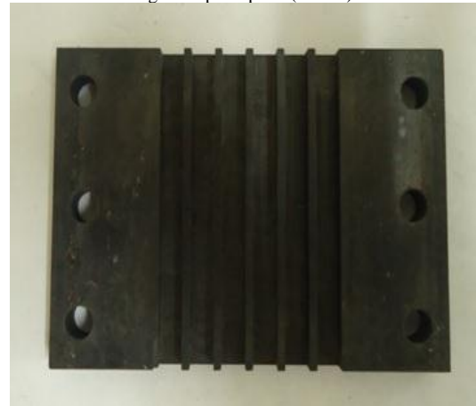
Fig.6 Cathode side graphite plate having parallel ducted flow channel
