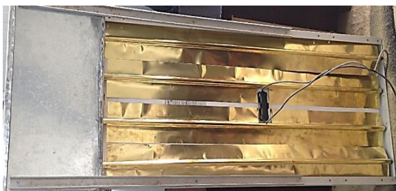
Fig. 13. Copper plate covering heat pipe and back of the panel [29]
