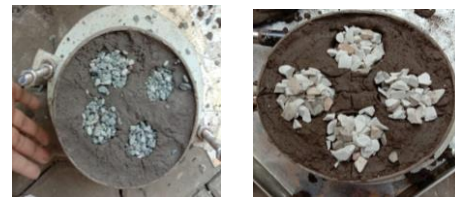
Fig 8 Square Pattern Arrangement of (a) Stone Columns (b) Ceramic Columns
