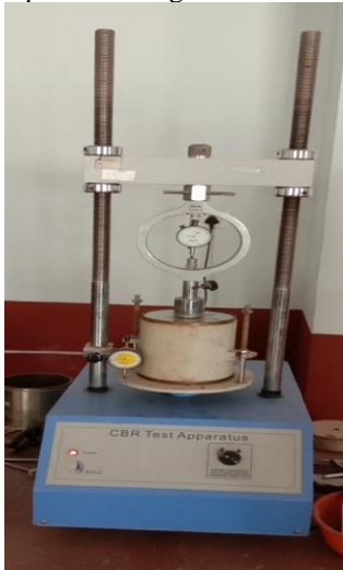
Fig 2 .Loading Using CBR Testing Machine
