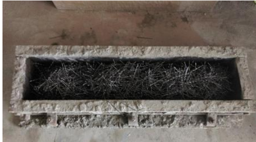
Fig. 3. Steel Fibers preplaced in mold
