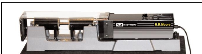
Fig. 1. Rotating bending fatigue test setup
