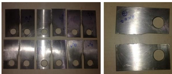
Fig. 5. Specimens after fatigue crack growth analysis
