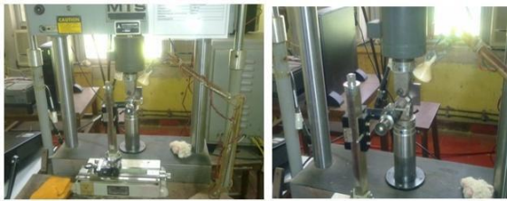
Fig. 4. Fatigue crack growth analysis setup
