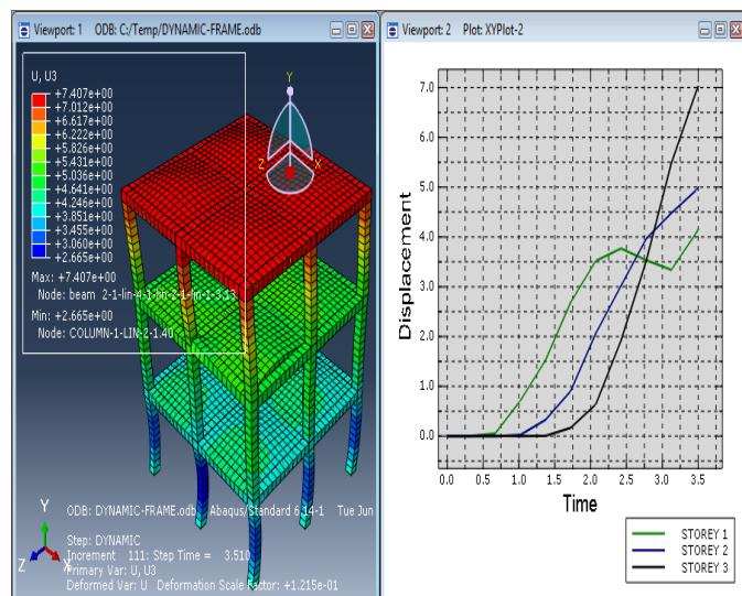
Fig.2 bare frame displacement curve
