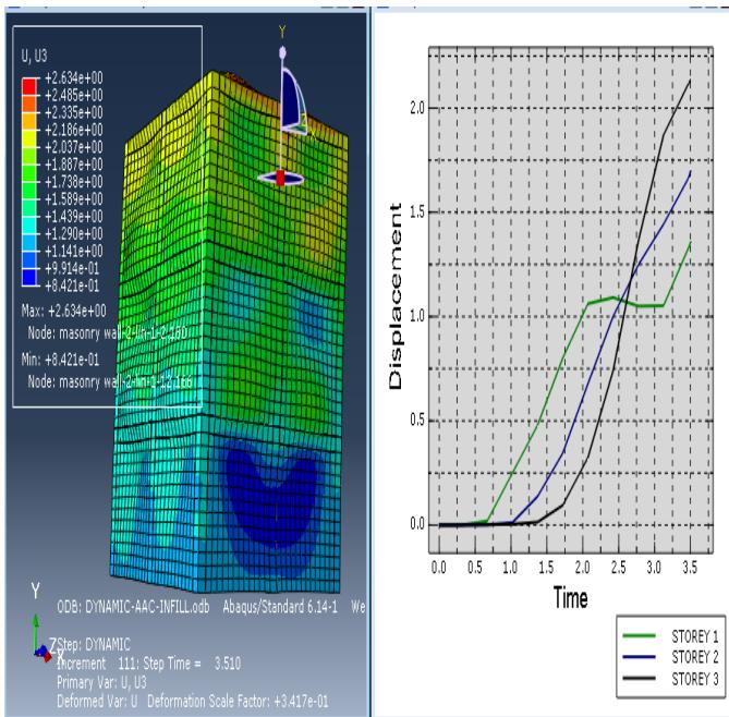
Fig.4 bare frame with conventional infill wall displacement curve
