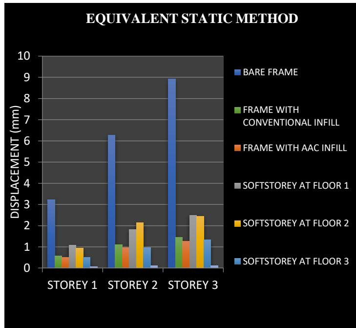
Fig.5 Story v/s Displacement graph
