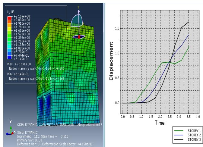
Fig.3 bare frame with AAC infill wall displacement curve
