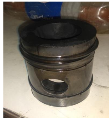
Fig 6. shows the hemispherical combustion chamber shape and having the 80mm bore diameter with 25mm radius.
