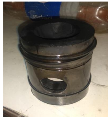
Fig 6. shows the hemispherical combustion chamber shape and having the 80mm bore diameter with 25mm radius.
