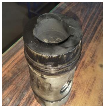
Fig 7. Cylindrical combustion chamber shape.
