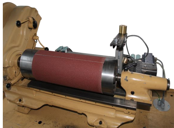
Fig 7(b). Pin on drum wear testing machine
