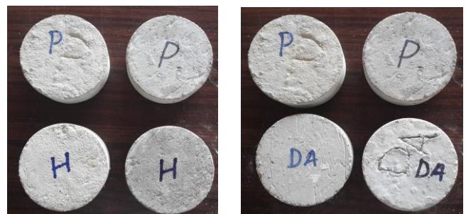
Fig.2. Typical M25 grade SCC concrete disc with different optimum % of organic corrosion inhibitors
