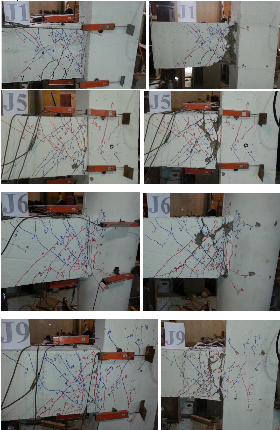
Figure (8) Cracks patterns and failure mode of joint (J1, J5, J6 and J9).
