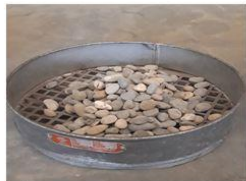
(B)Aggregate size 10-16mm
