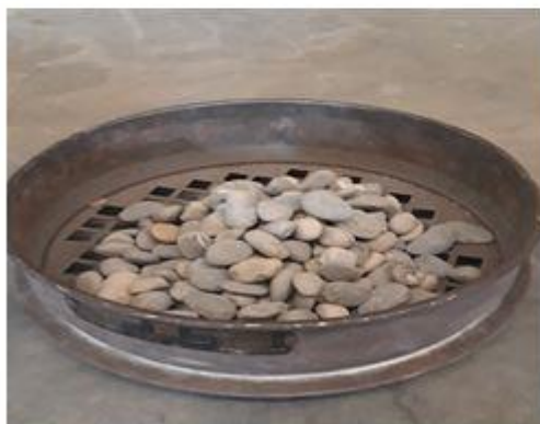
(C)Aggregate size 16-20mm
