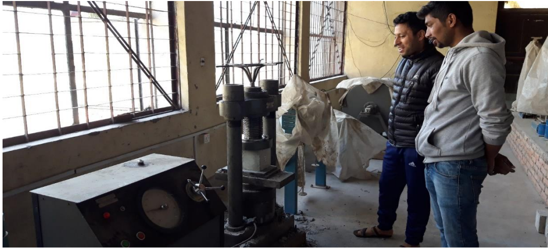
Fig. 3: Concrete Cube Under Compressive Strength Testing Machine
