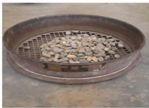
(A)Aggregate size 4.75-10mm
