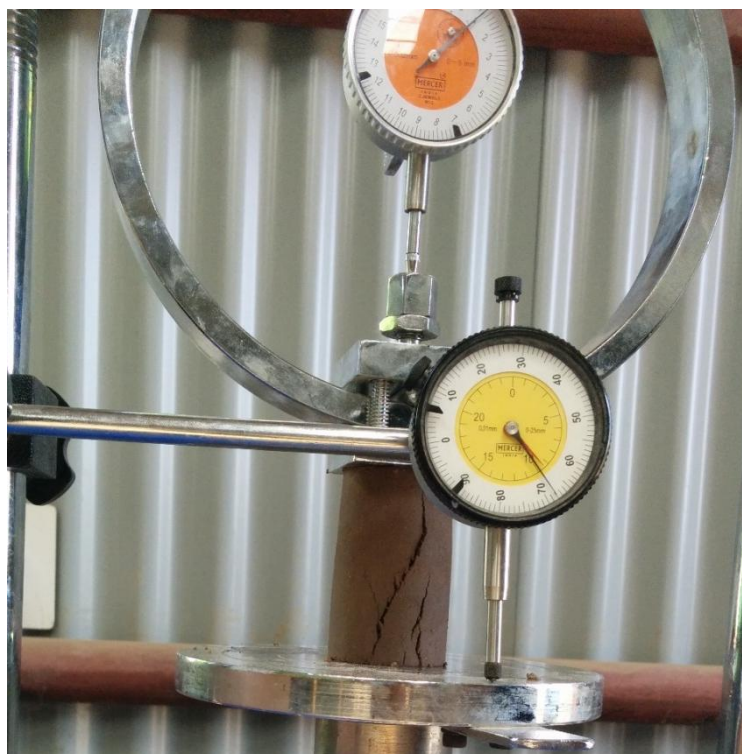
Fig. 1. Soil Sample under Unconfined Compression Testing Machine showing start of failure.
