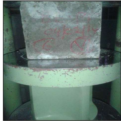
Figure 4: Compression Test on Concrete Cube
