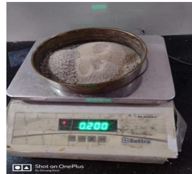
FIGURE NO: 1.1. Weighing of Ennore Sand.
