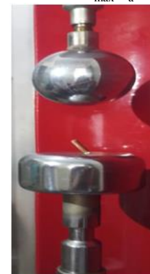
Figure 1: Sphere-Plane electrode arrangement.
