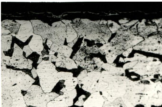
Fig. 1. Microstructure of the surface layer after titanization in the mixture № 5 (see Table 1), × 150: a – on low carbon steel; b – on gray cast iron.
