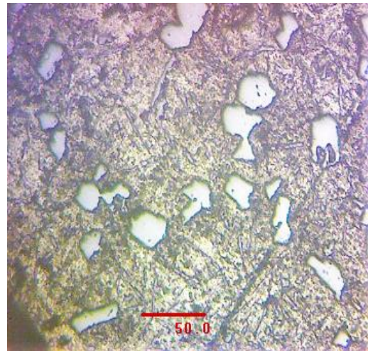
Fig 4: Microstructure of Al-18Si-2Cu.
