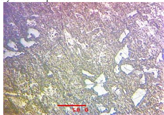
Fig 6: Microstructure of Al-18Si-2Cu-2Ni.
