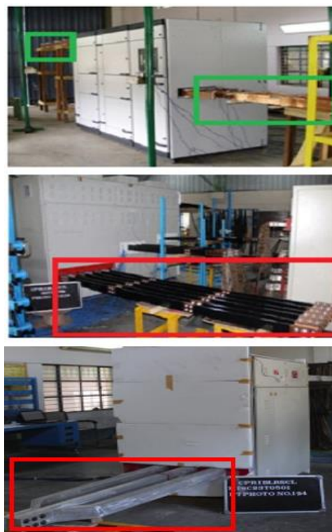
Figure.2 Configurations of Temporary test conductors
