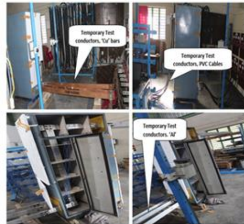
Figure.3 Test Set up with test conductors mounted
