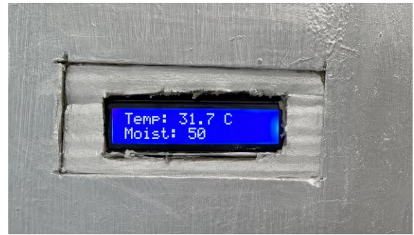
Fig-2: Display Panel of Composting System
