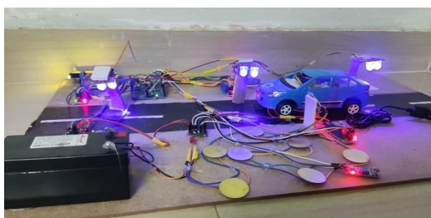
Fig.12.From the piezo electric energy the street lights are ON
