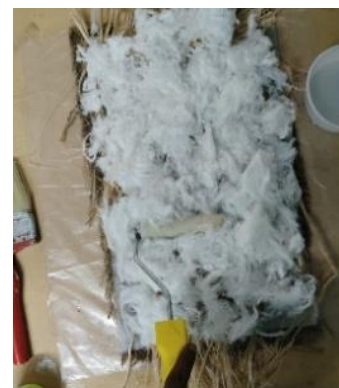
FIG 2 : HAND LAY-UP METHOD
