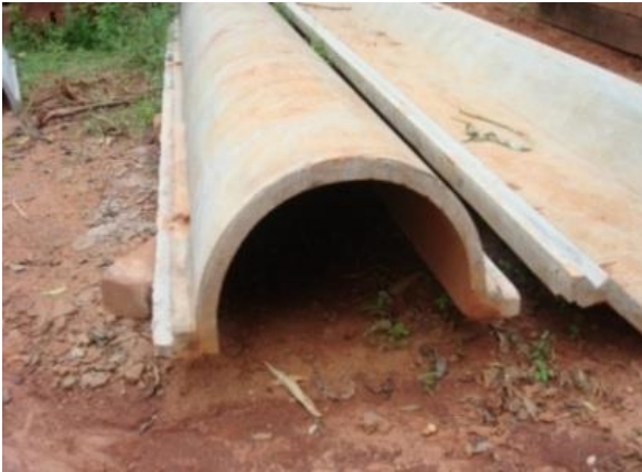
Fig:2 Precasted ferrocement hollow column
