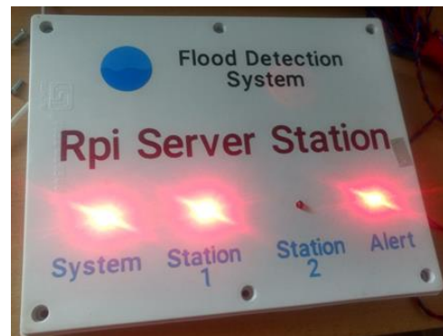
Fig. 13 Station 1 is at Flood Condition
