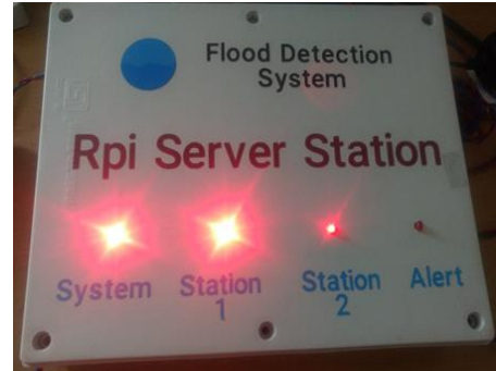
Fig. 12 At Normal Level of Both Stations
