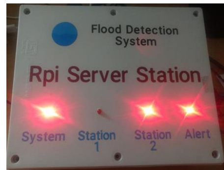
Fig. 14 Station 2 is at Flood Condition
