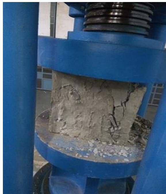
Fig 5: Failure of E-waste sample under load
