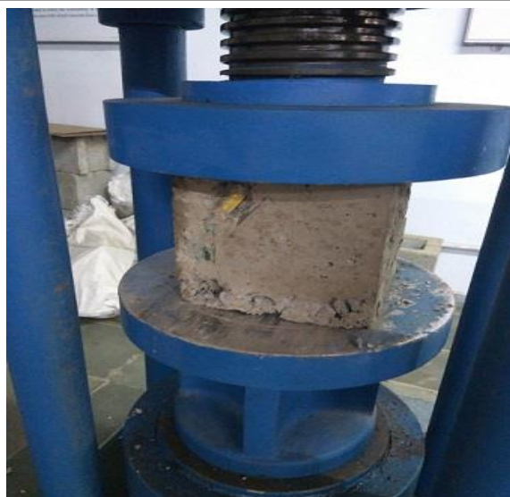
Fig 4: Testing of E-waste sample in CTM
