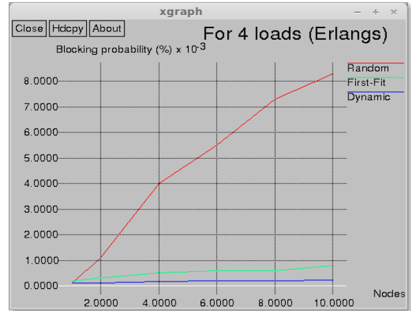
Figure 4: Blocking Probability (%) with four Erlangs for random fit, first fit and proposed conversion
