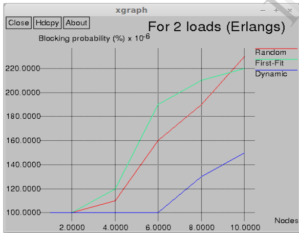
Figure 3: Blocking Probability (%) with two Erlangs for random fit, first fit and proposed conversion
