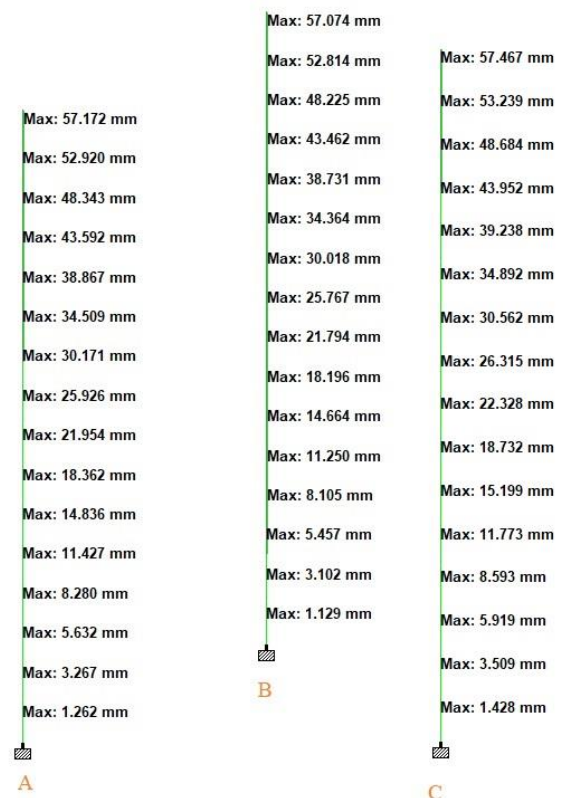
Figure 13. Displacement of Type B Building.
