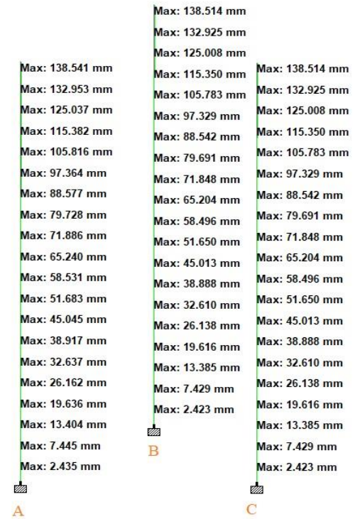
Figure 15. Displacement of Type D Building.
