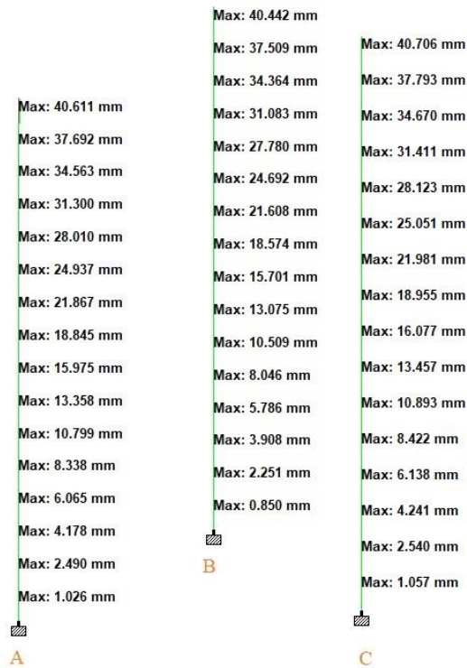
Figure 14. Displacement of Type C Building.
