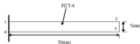
Fig 4.1. Model of simple beam made of piezoelectric (PZT-4)
