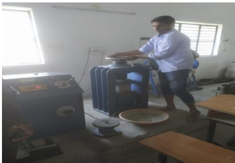
Fig 2: Testing cubes under UTM machine
