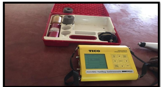
Fig-4: Ultrasonic Pulse Velocity Test
