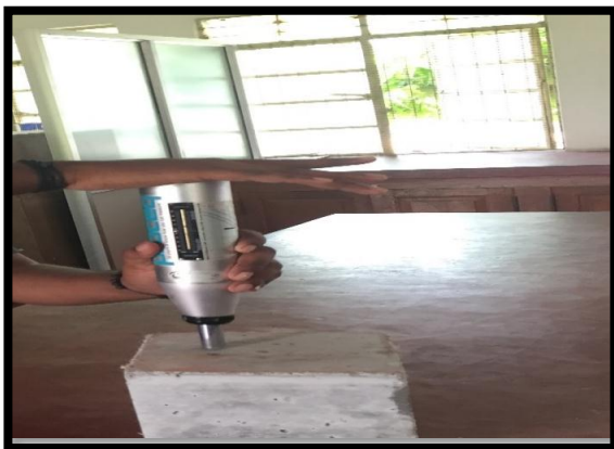
Fig-3: Rebound Hammer Test
