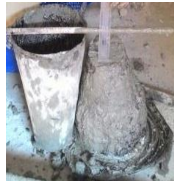
Fig.2.3 Slump test on M20 grade of concrete
