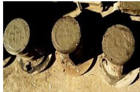
Fig.2.4 Casting of Cylinder
