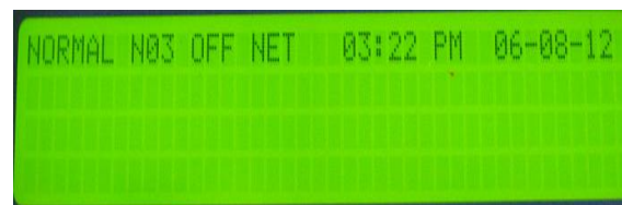
Fig: 11.b. Node 3 panel's display with off net status when not in network
