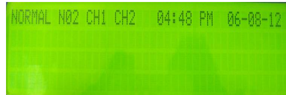
Fig: 10.b Node 2 panel's display with on net status when in network
