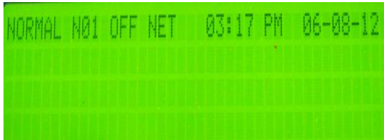
Fig: 9.a. Node 1 panel's display with off net status when not in network
