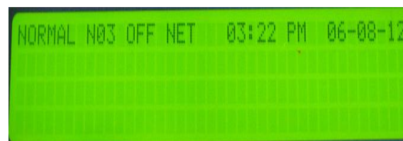
Fig: 11.c. Node 3 panel's display with off net status when not in network
