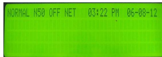
Fig: 11.a. Node 50 panel's display with off net status when not in network
