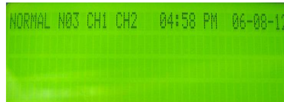
Fig: 10.c Node 3 panel's display with on net status when in network
